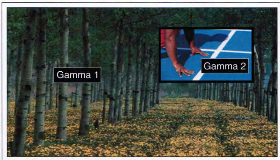
Fig. 4: In the PPDS™ architecture, the gamma tables that reside in the timing controller allow picture-in-picture windows to have different gamma mappings, so colors can be optimized separately for each image.
